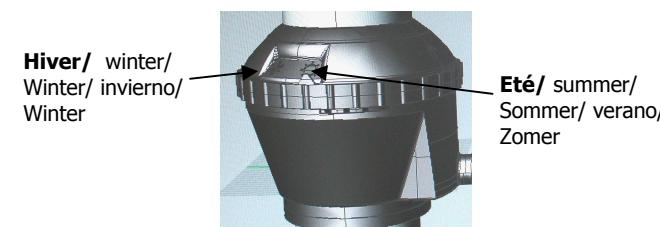
Care, the filling system of the tank works only if the kit placed on the rain pipe, is on position "openned". Position called "summer", symbolized by the "sun". Conversely, in order to stop the filling, put the kit on position "closed", symbolized by the "ice crystal".
