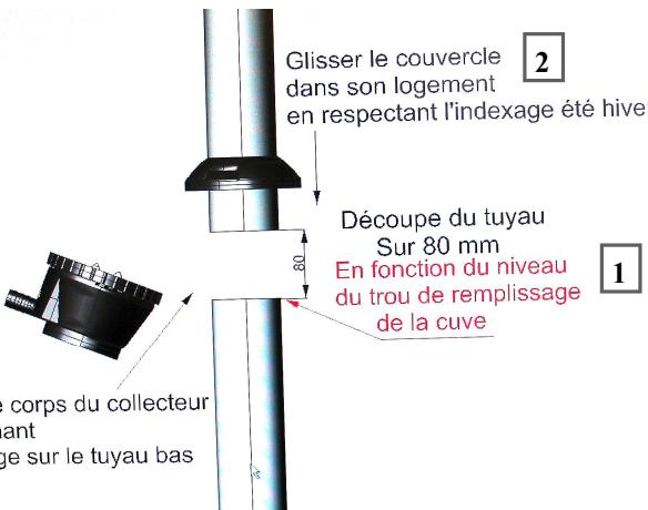
3/ Saw the down pipe at equal height to the maximum level water.
