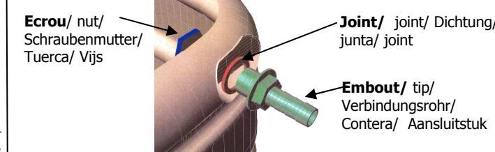
1/ Bore the hole of filling (materialised on the tank) on the adequate side and refine it taking away burrs. Then connect the connecting tips on the tank.
