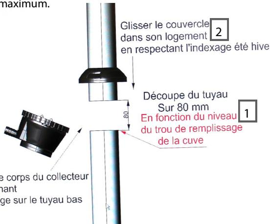
3/ Saw the down pipe at equal height to the maximum level water.
