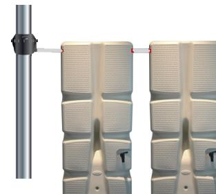
It is enough to place one second tank on the first. You need for this: 1 pipe Ø 20mm interior + 2 connector tips. Bore the filling hole opposite to the one connected to the collector and bore also the filling hole on the second tank. Put the connecting tips on the both tanks and connect them with the pipe.
